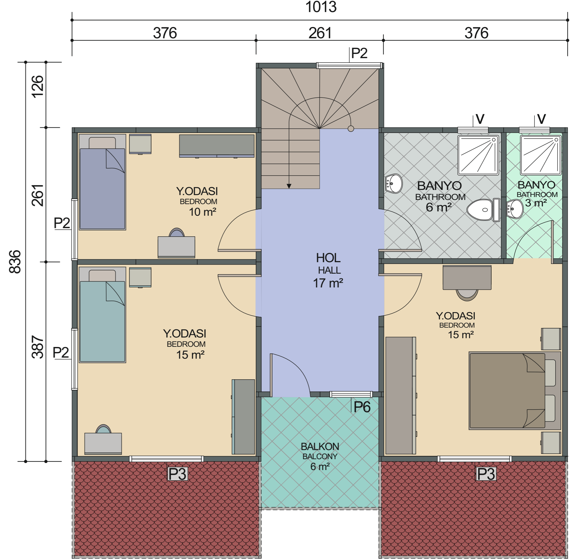
1. KAT PLANI FIRST FLOOR PLAN 66 \text{ m}^2 + 6 \text{ m}^2 = 72 \text{ m}^2
